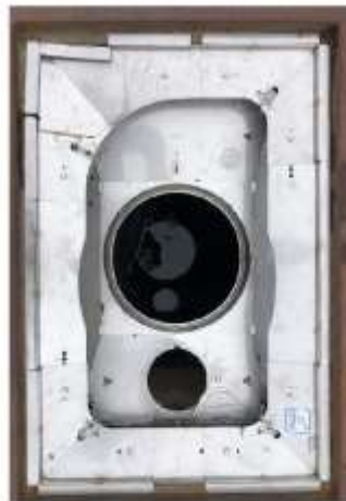
Image 4 - top view of Device with Mundus Bag removed and sample port open that shows catch basin access
