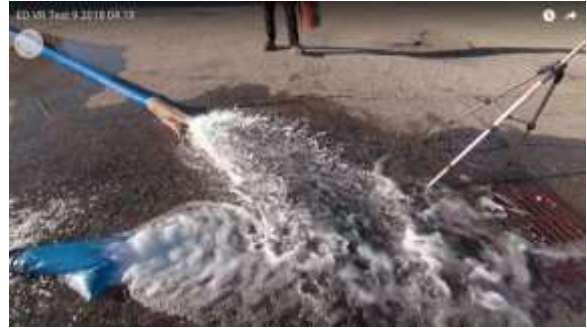
Image 22 - 500 gpm test of Device showing trash entering Device
