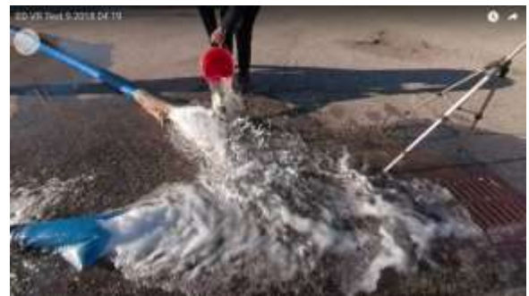
Image 20 - 500 gpm test of Device. Introducing simulated trash recipe
