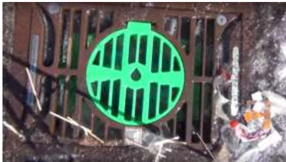
Image 23 - Device equipped with optional OGB grate during a 350 gpm test
