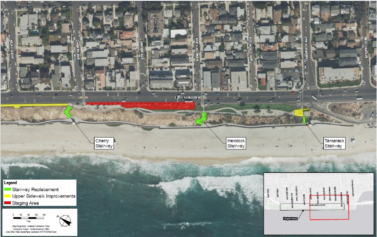
Figure 3 : Beach Access Repairs Project Overview
