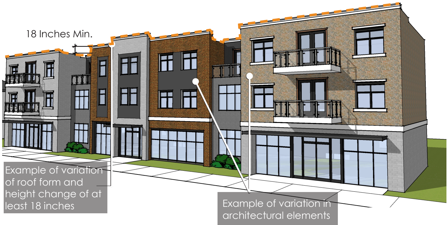
Figure 7: Rooflines shall not extend horizontally more than 40 feet in length without a prominent change in roof form, variation in architectural elements, or a variation in roof height (3.A.4)
