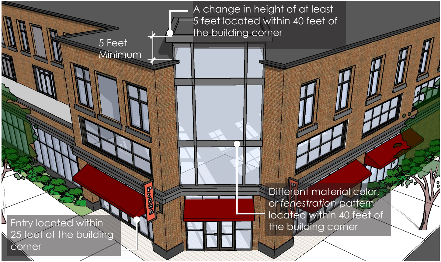
Figure 6: Corner buildings shall incorporate a building entrance, variation in materials, colors, or fenestration, or a variation in height (3.A.3)
