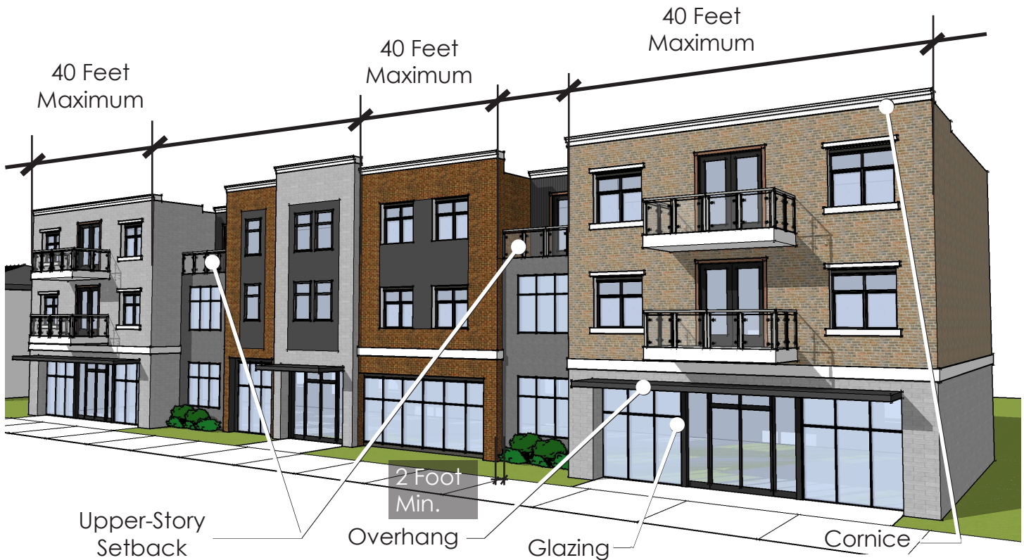
Figure 5: Building facades shall not extend horizontally more than 40 feet in length without a variation in the wall plane (3.A.2)
