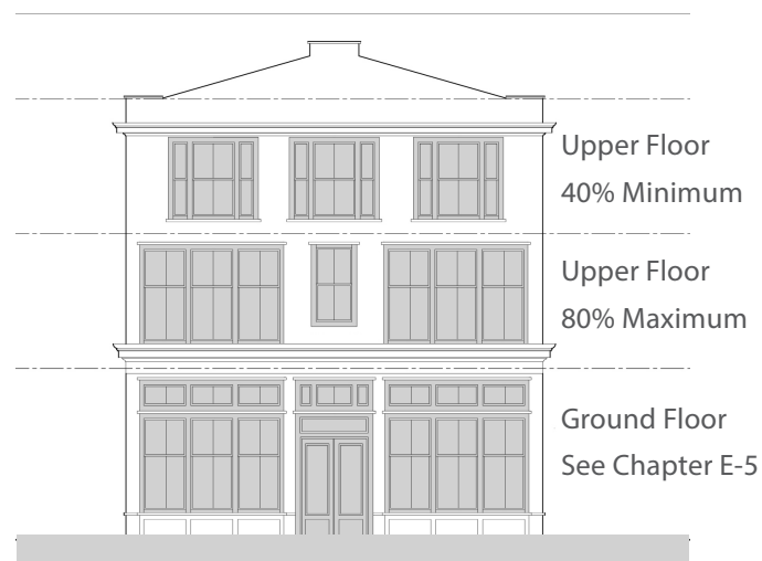
Figure 6.3 Facade Transparency Upper Floors - Mixed Use
