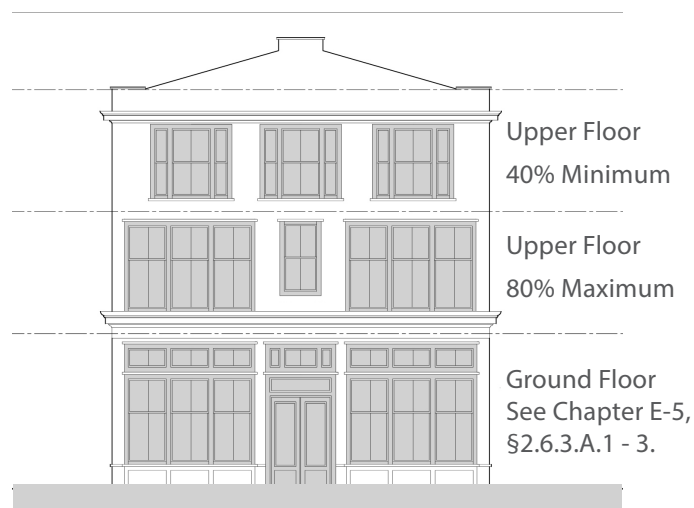
Figure 6.2.3 Facade Transparency Upper Floors - Mixed Use
