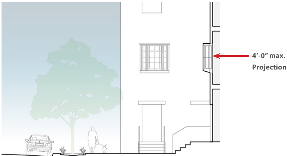
Figure 6.3.5 Bay Window Section
