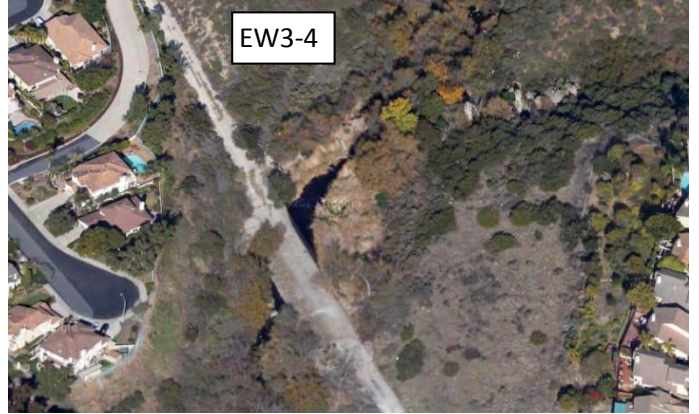
EW3-4. Unnamed road crossing San Marcos Creek; may be abandoned or used for maintenance. Does not appear to obstruct movement (at grade crossing), but this should be confirmed in the field if possible.
