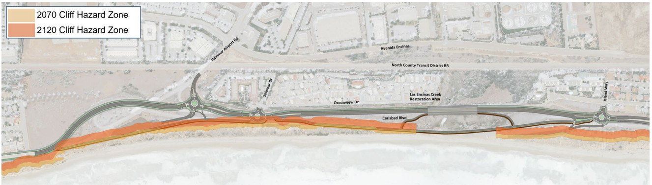
Figure 6. Cliff Hazards in the Project Area with Sea Level Rise Projections for 2070 and 2120
