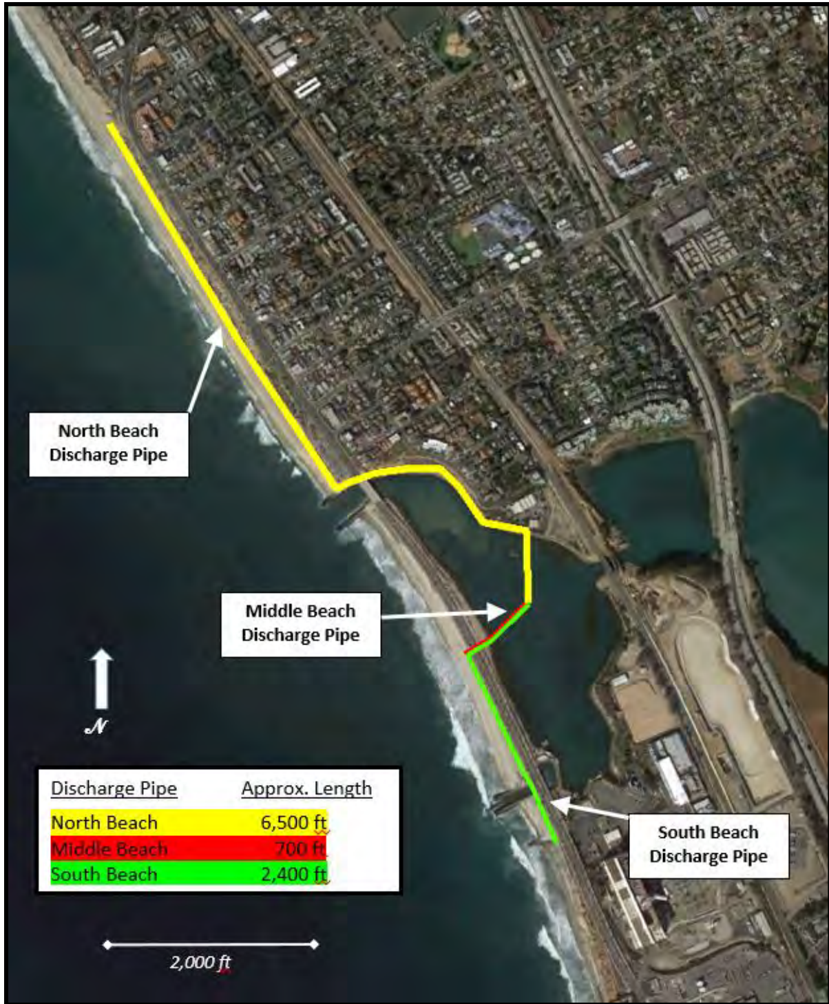
Figure 2. Dredge Discharge Pipeline Routes
