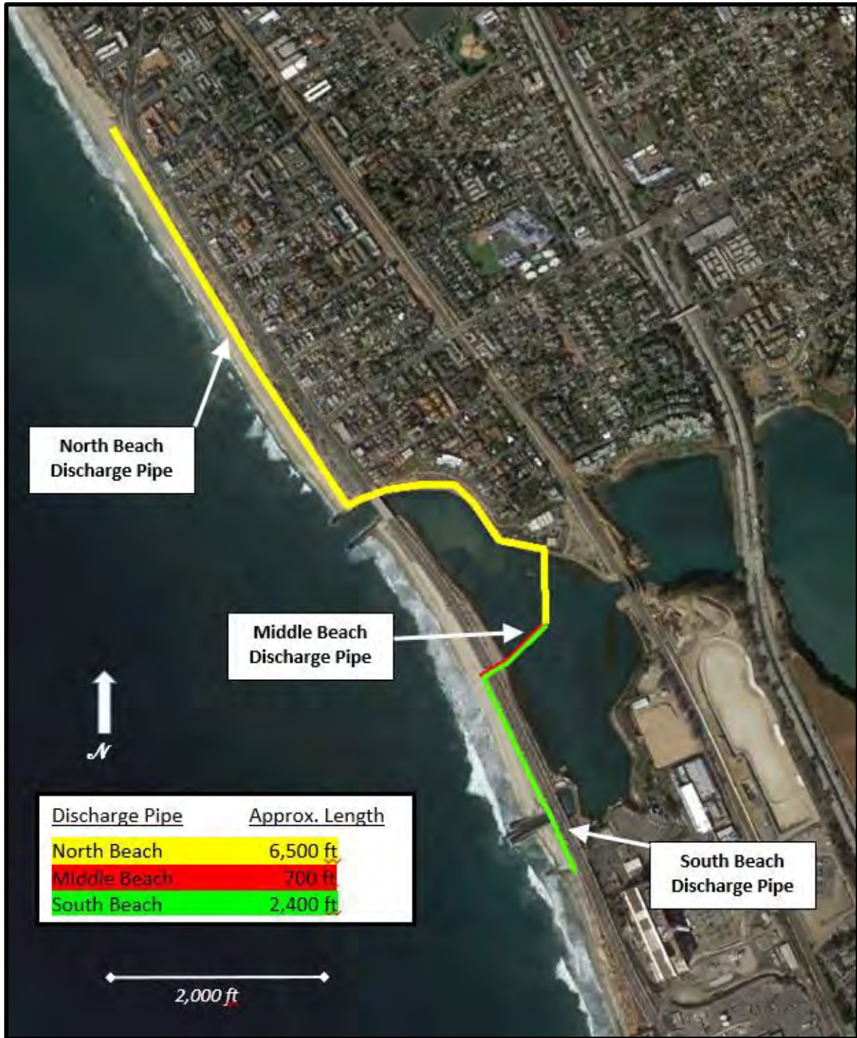
Figure 2. Dredge Discharge Pipeline Routes
