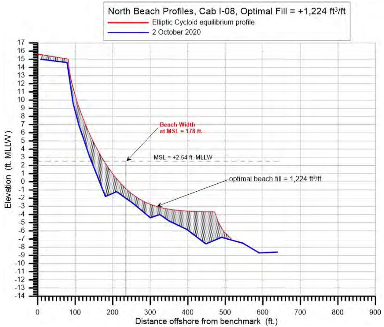
Figure D-8: Permitted beach fill at range line Cab I-08 on North Beach based on fill distribution as elliptic cycloid equilibrium profiles.
