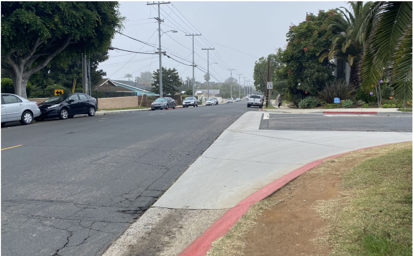
Wide right turn turning radius and absence of crosswalks at the intersection of Jefferson Street and Chinquapin Avenue.
