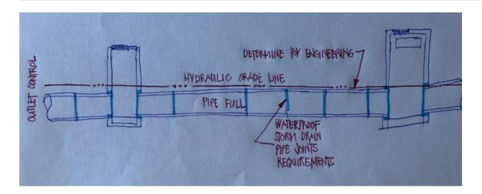
I suggest the Conditions of Approval require all storm drain conduits below the hydraulic grade line have joints sealed or alternative to add pipe lining with new technology.
