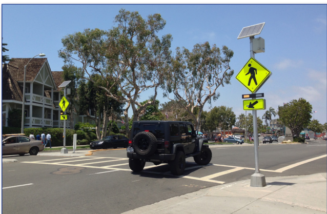
Multiple lanes require positive protection such as this Rectangular Rapid Flashing Beacon
