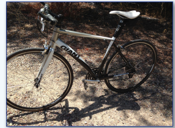
A hybrid commute bike with thinner tires is considered to be the minimum requirement to determine if the trail is usable as a transportation asset. This type of bike can handle firm surface compacted trails but cannot handle the soft surfaces that a wide, medium pressure tire of a mountain bike can handle.
