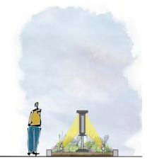
Figure 67 – Sign lighting, bullet luminaires with snoots for glare control
