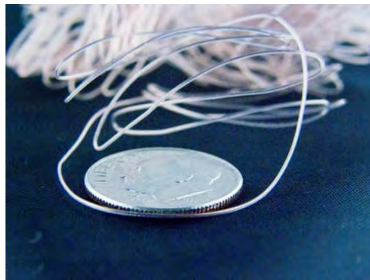
Figure 17 CEW cartridge wire (127 microns) and U.S. dime.
