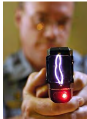
Figure 24 Illustrating CEW Drive-Stun Discharge Across Front Electrodes and LASER.
