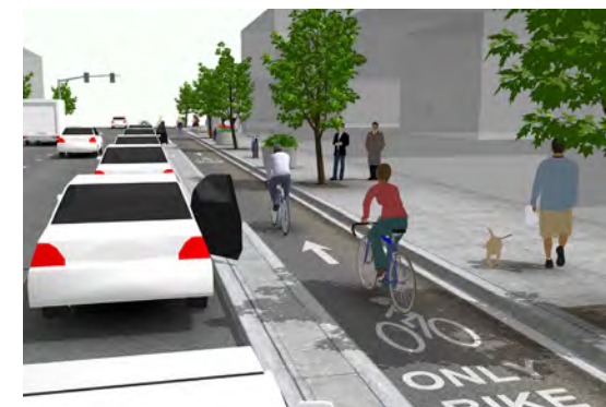
One-Way Class IV Cycle Track. (Source: NACTO)
