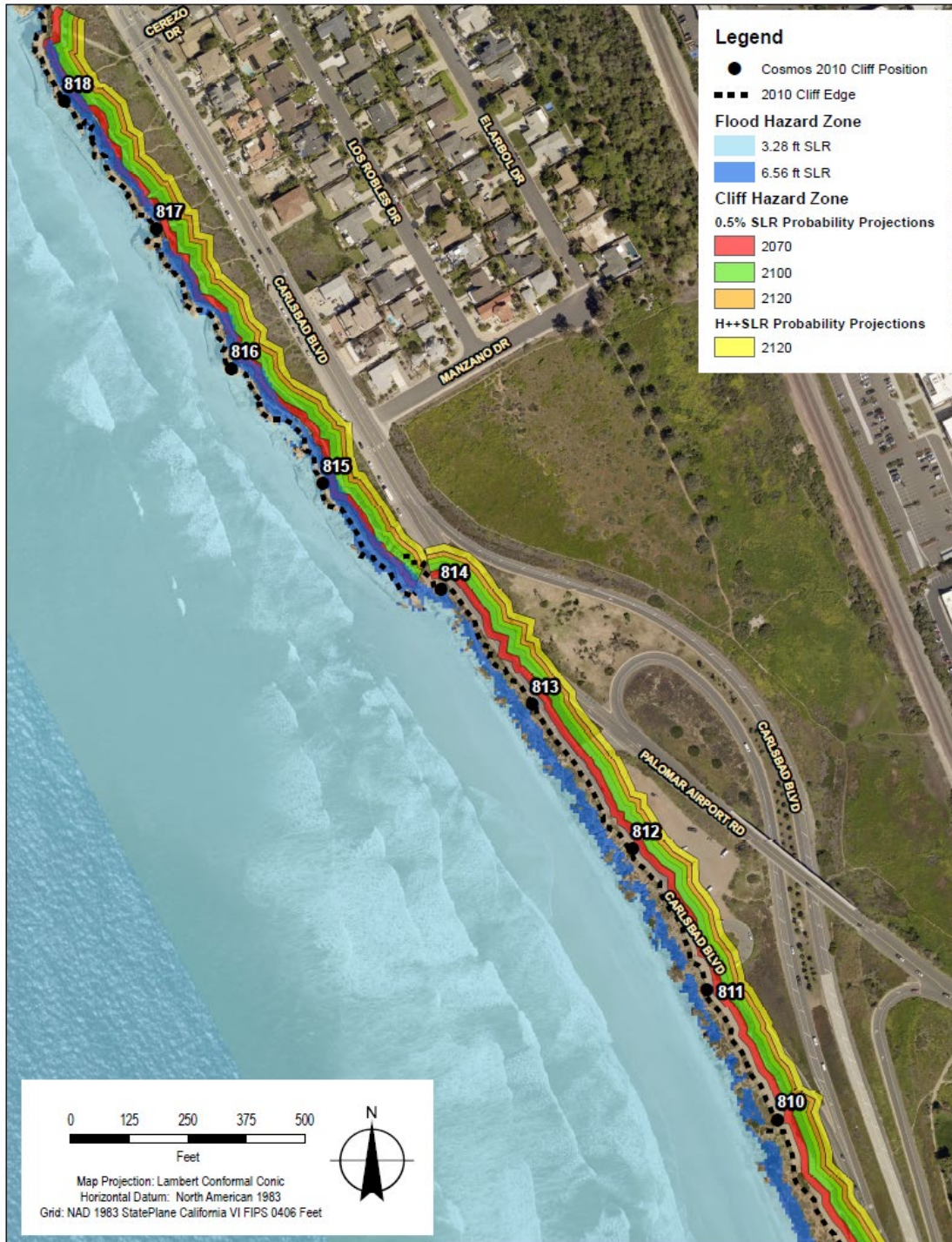
Figure 4-1. Interim Coastal Hazards in the Northern Project Area
