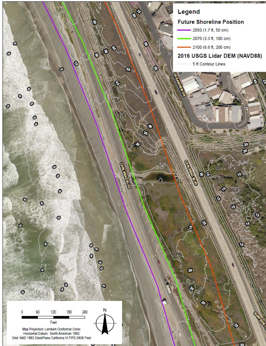
Figure 2-1: CoSMoS COAST Future Shoreline Position assuming Exiting Revetment Removal
