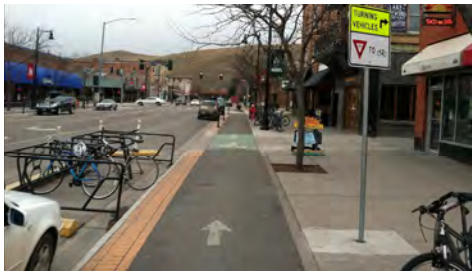
A raised cycle track in Bozeman, MT provides a similar scale precedent to the one proposed for Carlsbad Village Drive.
