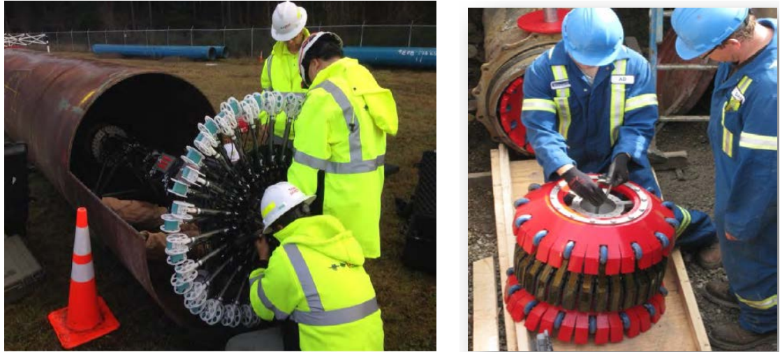
Figure 3-22. Example of In-Pipe Electromagnetic Technology
