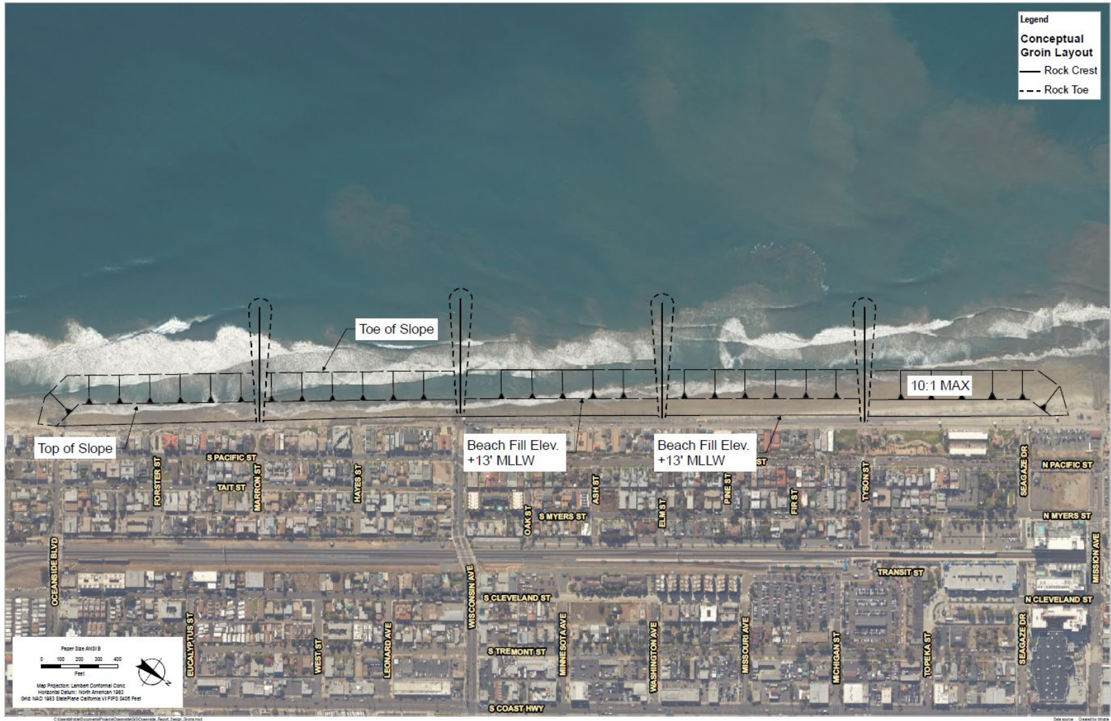
Figure 6-2. Groin Field Concept
