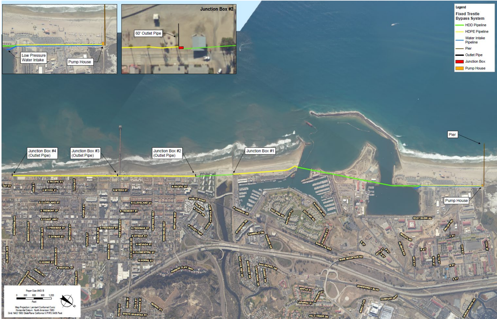
Figure 11-1. Fixed Trestle Sand Bypass Option
