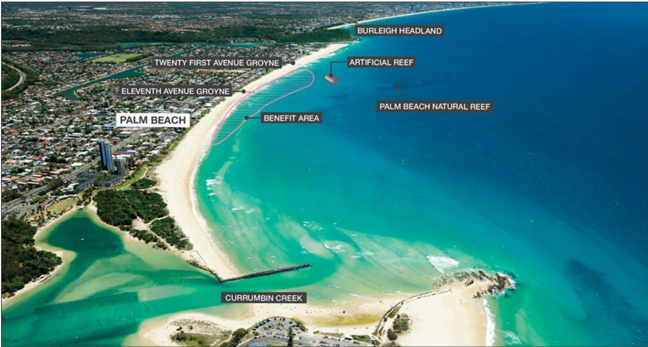
Figure 2-16. Palm Beach Artificial Surf Reef (Source: City of Gold Coast, 2019)
