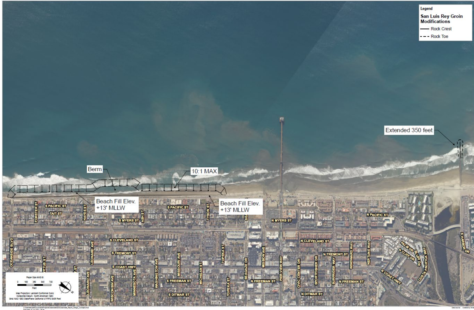
Figure 6-3. San Luis Rey Groin Extension Concept
